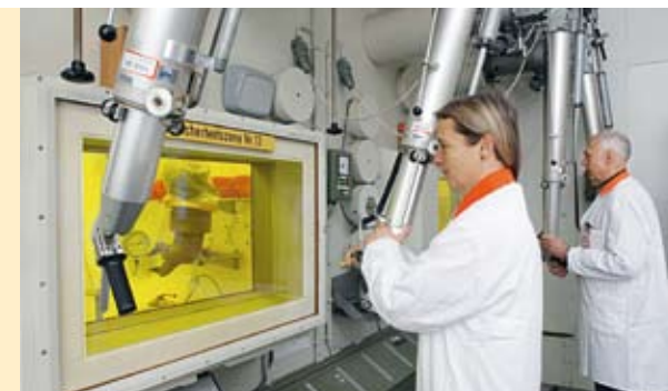
Disposal technology Decontamination of nuclear graphite
