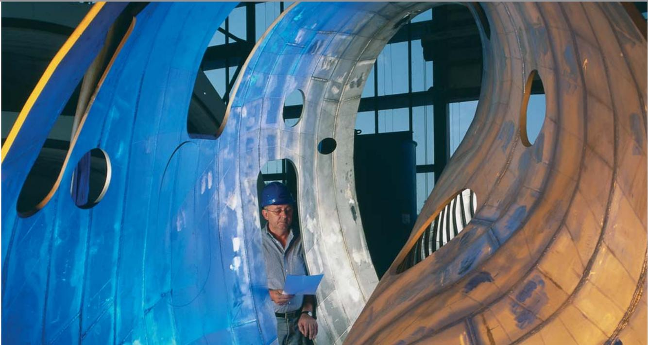
TEILSTÜCK DER PLASMAKAMMER DES FUSIONSEXPERIMENTES WENDELSTEIN 7-X: ZWANZIG DIESER ELEMENTE WERDEN ZU EINEM RING ZUSAMMENGEFÜGT. Foto: IPP/W. Filser
