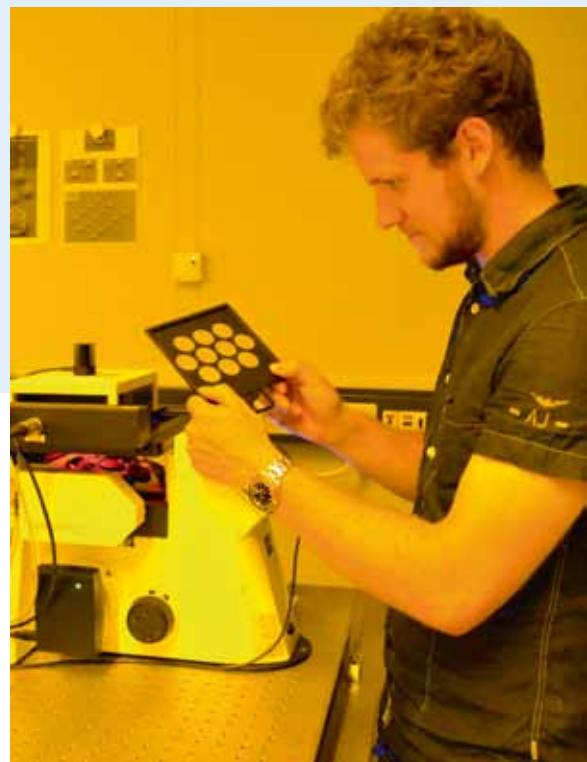
Diploma candidate Tiemo Bückmann loading the dip-in laser writing device that is used to generate the desired metastructures in the material. Photo: CFN/KIT
