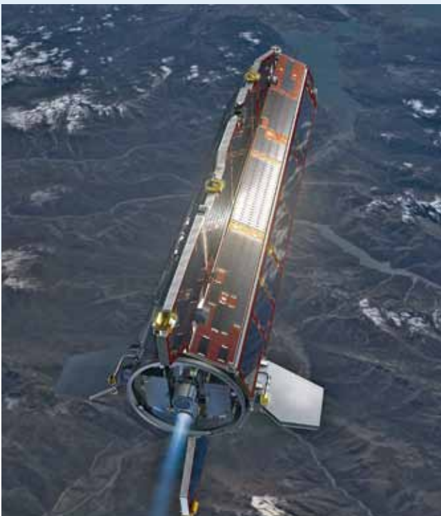
ESA's 5.3-metre GOCE satellite flies in a sun-synchronous polar orbit at an altitude of about 260 kilometres taking measurements of the Earth's gravitational field. Photo: ESA/AOES Medialab
