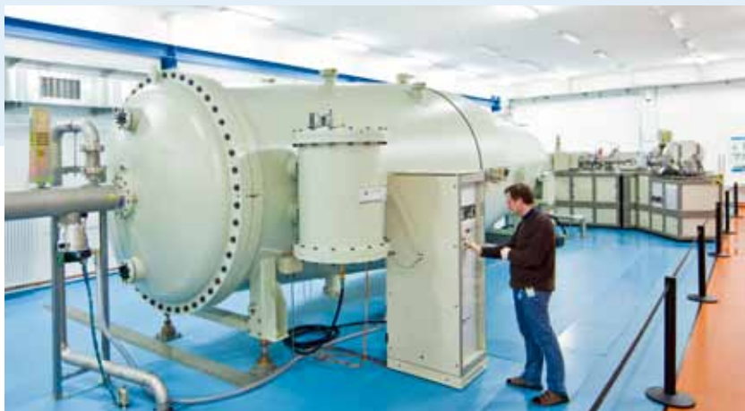
In order to produce quantum dots from indium arsenide, researchers use the ion accelerator at the HZDR’s ion radiation centre. The photo shows the six-megavolt ion accelerator, which was funded by the EU as part of the EFRE programme. Photo: Oliver Killig/HZDR
