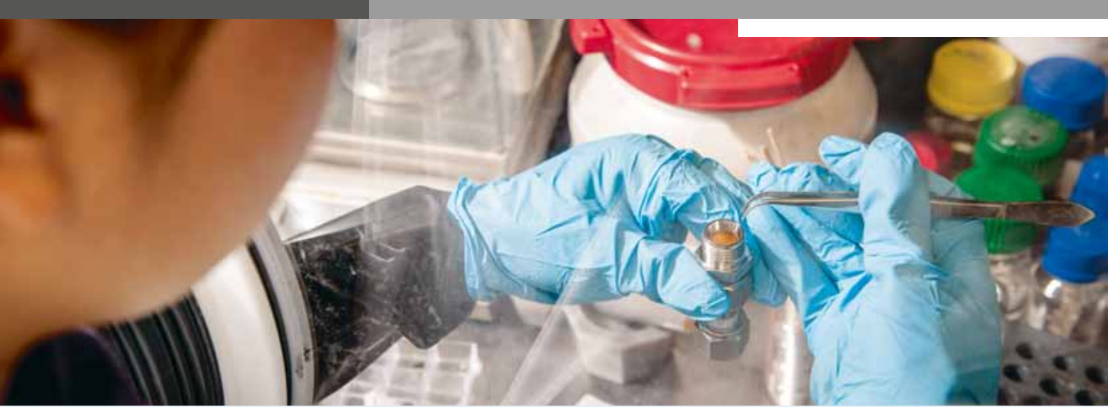
A scientist assembling a test cell in a glove box with an inert gas atmosphere that prevents unwanted reactions. Photo: KIT
