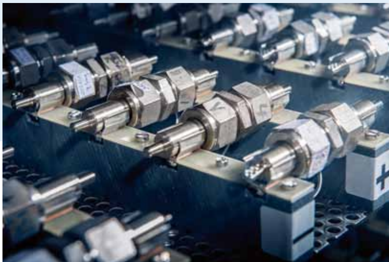
Battery cells being tested under controlled temperature conditions. Photo: KIT
