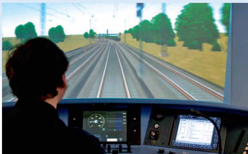
The DLR's RailSET railway laboratory allows researchers to carry out technical and operational tests for train trips. Photo: DLR
