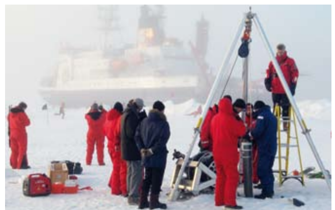
AUTONOMOUS MEASURING BUOYS THAT TRANSMIT DATA VIA SATELLITE WERE DEPLOYED IN THE CENTRAL ARCTIC DURING AN EXPEDITION OF THE POLARSTERN RESEARCH VESSEL IN 2007. Photo: Karel Bakker/NIOZ
