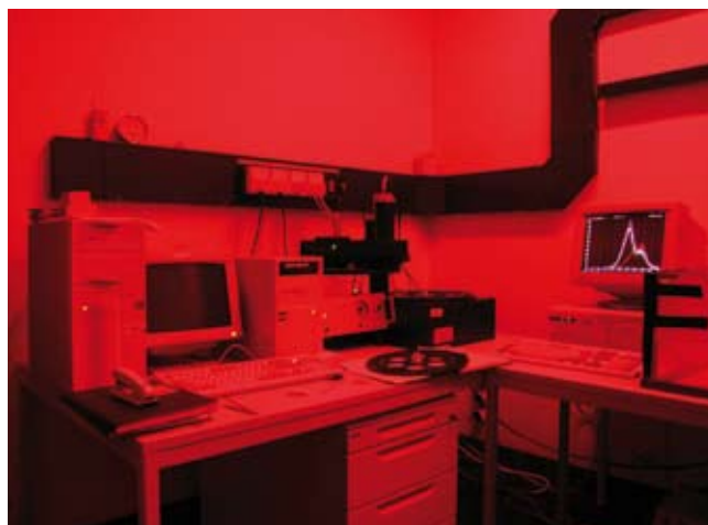
LUMINESCENCE MEASURING OF BRICK SAMPLES ENABLE THE RECONSTRUCTION OF EARLIER RADIATION EXPOSURE. Photo: Helmholtz Zentrum München/Y. Gösku
