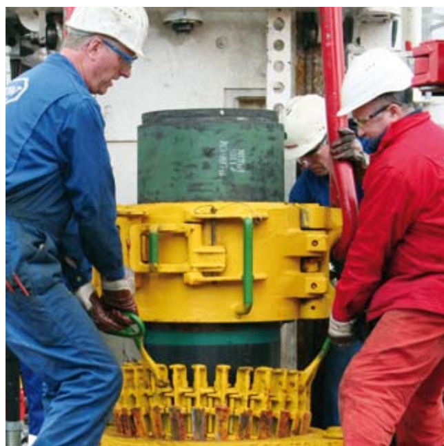
PIPES ARE NEEDED FOR THE LONG-TERM STABILISATION OF DRILL HOLES THAT ARE SEVERAL KILOMETRES DEEP. Photo: GFZ
