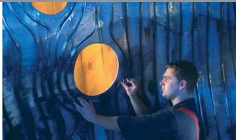
ITS SHAPE CLOSELY FOLLOWS THE INTRICATE CONTOURS OF THE PLASMA. PORTS PROVIDE ACCESS TO THE PLASMA FOR HEATING AND MEASUREMENT DEVICES. Photos: IPP/W. Filser
