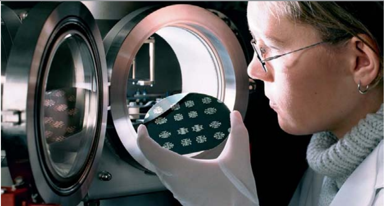
WORKING AT PETER GRÜNBERG'S LABORATORY, A RESEARCH ASSISTANT PUTS THE FINISHING TOUCHES TO THE SANDWICH STRUCTURES (ON THE WAFER). Photo: FZ Jülich
