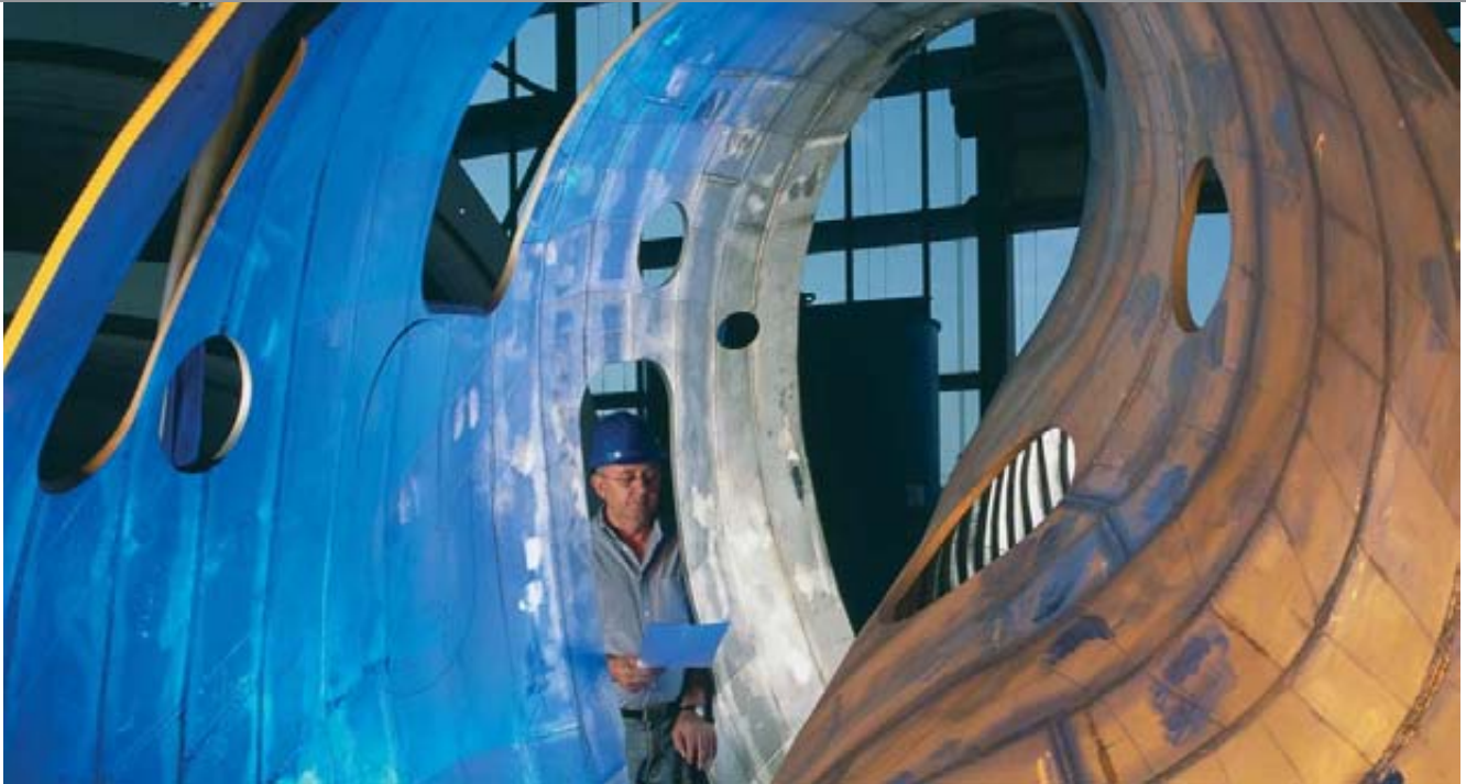
PART OF THE PLASMA CHAMBER FOR THE FUSION EXPERIMENT WENDELSTEIN 7-X: TWENTY SUCH ELEMENTS ARE JOINED TOGETHER TO BUILD EACH RING. Photo: IPP/W. Filser
