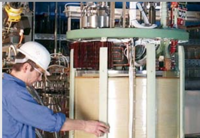
SUPERCONDUCTING HIGHEST FIELD MAGNETS EXAMINED THOROUGHLY ON THE HOMER 2 TEST BED AT THE INSTITUTE FOR TECHNICAL PHYSICS. Photo: Forschungszentrum Karlsruhe
