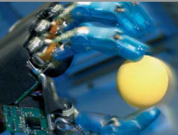
THE SENSITIVE HANDS EVEN HOLD SOFT OBJECTS. Photo: DLR
