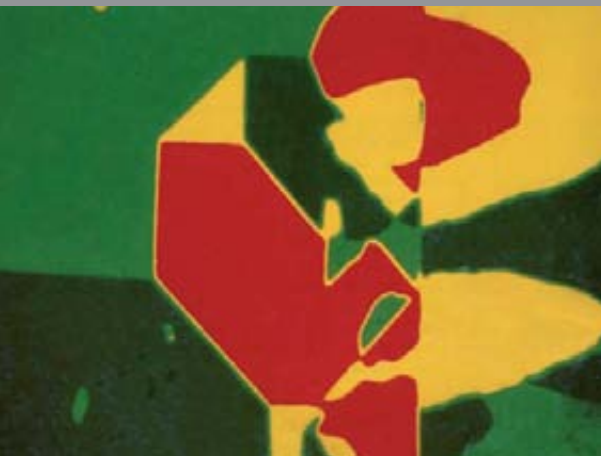
THE VARIOUS MAGNETIC DOMAINS OF THE MICROSANDWICH ARE CLEARLY RECOGNISABLE IN THE FALSE COLOUR IMAGE. Photo: FZ Jülich
