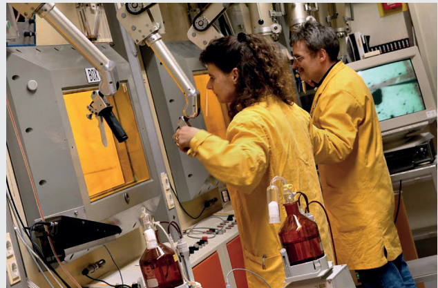
Thick lead glass panes protect the experimenters from the radiation of the radioactive samples. The KIT operates the currently largest German testing field for the decommissioning of nuclear installations. Foto: M. Breig/KIT
