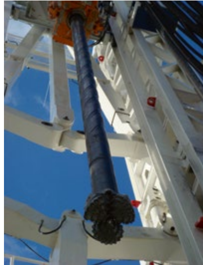
The InnovaRig deep drilling rig (left) and the rotary bits on the head of the drill pipe. Photos: GFZ
