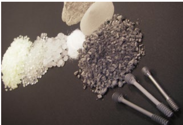
Metal powder injection moulding: top, the metal powders, to the left, the polymer components, and in the centre, the mixed granulate. Below: component precursors and, to the right, the completed Mg-Ca-bone screw. Photo: M. Wolff/HZG
