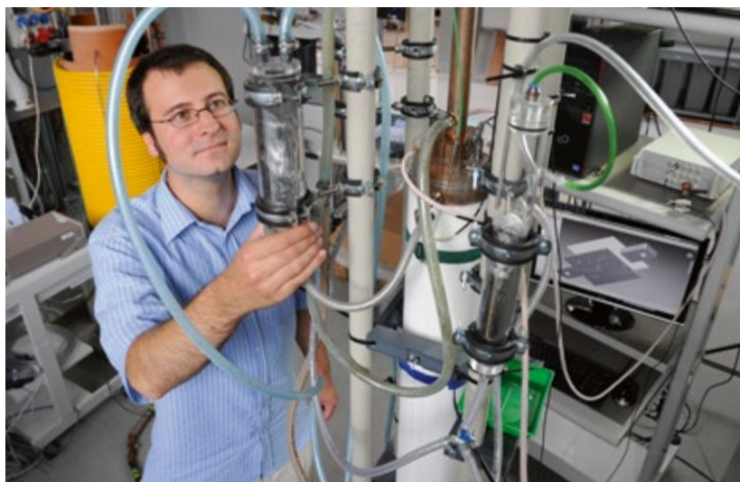
The Taylor instability slows down neutron stars in space; in large liquid metal batteries it can cause short circuits. Scientists first demonstrated this magnetic phenomenon in the laboratory using this experiment array at the HZDR – pictured here with doctoral candidate Marco Starace. Photo: Frank Bierstedt/HZDR
