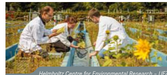
Scientists are using 47 artificial streams to study the effects of pesticides on flowing waters and the species living in them. Photo: Künzelmann/UFZ
