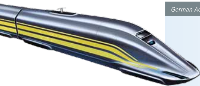
Flexible rail concept: the individual wagons are combined with one or two end cars to form a complete locomotive. Photo: DLR
