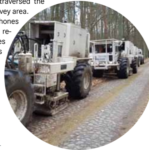
The 21-ton vibrator vehicles produced seismic waves that were recorded by geophones. Photo: GGD
