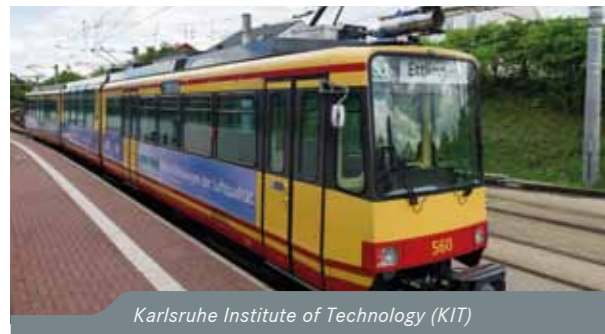
The light rail vehicle with the AERO-TRAM logo and the set of instruments over its cab has made a total of 6,228 test trips in Karlsruhe. Photo: Patrick Langer, KIT
