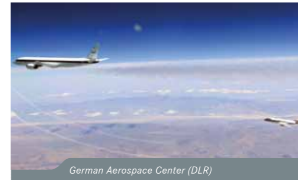
Scientists on board the DLR Falcon measured the composition of exhaust gas from the DC-8. Photo: NASA
