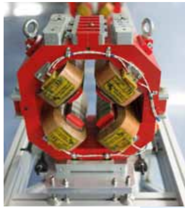
These quadrupole magnets were produced in the Budker Institute in Novosibirsk. Photo: M. Setzpfand/HZB
