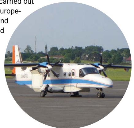
With its rectangular cabin and large floor openings, the twin-engine turboprop Do 228-212 aircraft is particularly well suited for the use of the special camera and radar systems. Image: DLR (CC BY 3.0)
