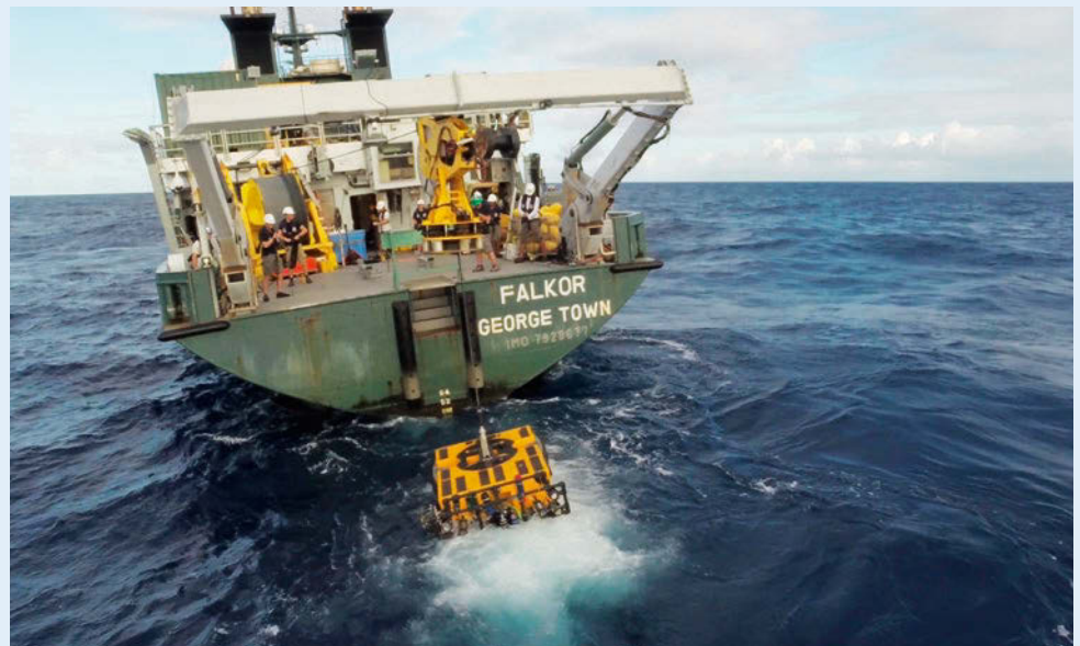
The ROPOS deep sea robot on its way to the ocean floor with the camera system developed at GEOMAR. Image: Björn Kurtenbach
