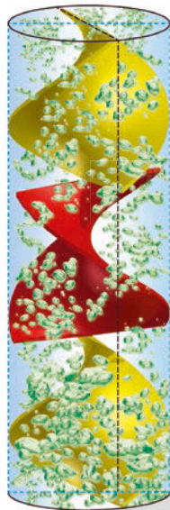
Static mixers like the one shown in this picture mix fluid flows directly in pipe systems. Image: Michael Voigt/HZDR
