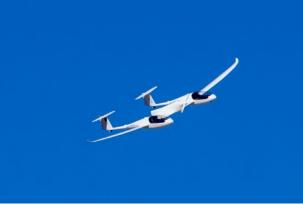
$\rm HY4$  - first four-seater passenger aircraft powered solely by a hydrogen fuel cell battery system (DLR)
