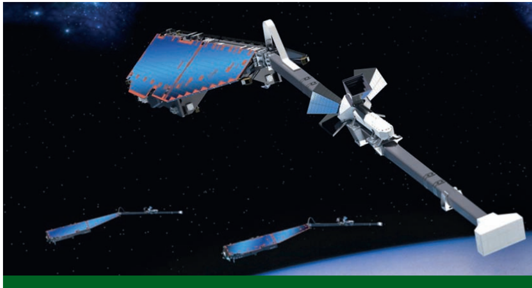
The three satellites of the SWARM mission are designed to measure the Earth's magnetic field starting in mid-2012.
