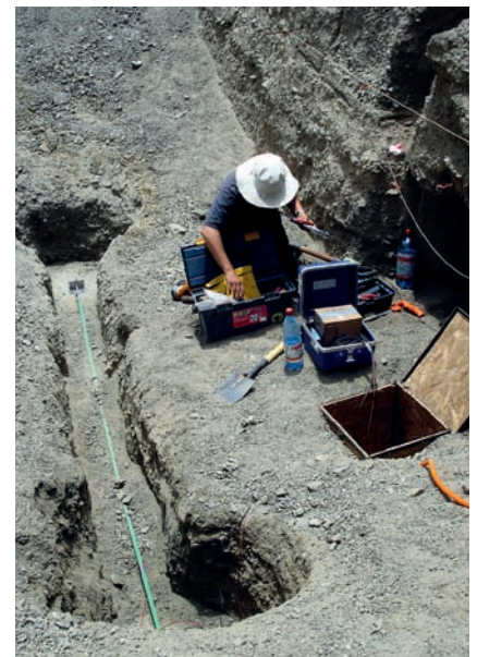
A creep meter in northern Chile measures tectonic shifts with unparalleled precision.
