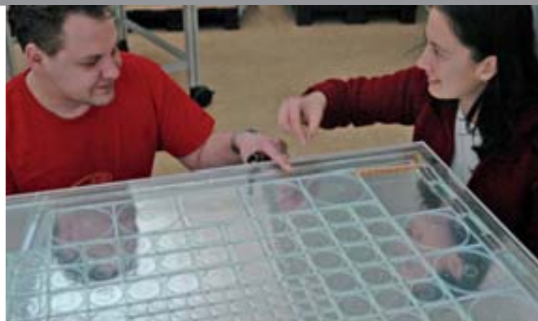
ONE OF 40 LAYERS FOR A PROTOTYPE ENERGY SENSOR: THE "EYES" ARE MADE OF PLASTIC DISKS THAT CONVERT PARTICLE ENERGY INTO LIGHT. Photo: DESY
