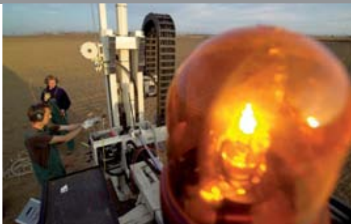
CONCENTRATION-DEPTH PROFILES OF SELECTED SUBSTANCES IN GROUNDWATER ARE MEASURED USING A DIRECT-PUSH MACHINE. Photo: Künzelmann/UFZ
