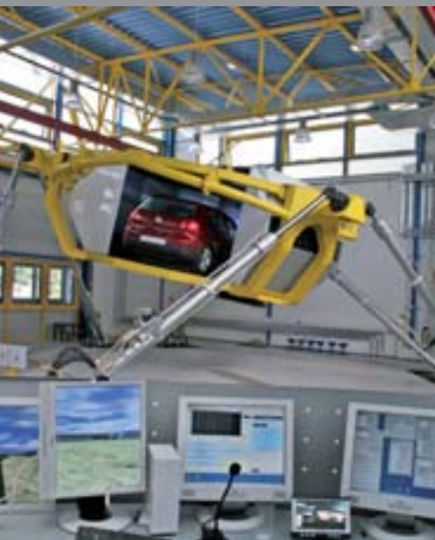
A DRIVING SIMULATOR HELPS PSYCHOLOGISTS TEST HOW ASSISTANCE SYSTEMS SUPPORT DRIVERS. Photo: DLR
