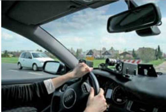
A CAMERA RECORDS THE DRIVER'S ACTIONS AND LINE OF VISION WHILE TRAVELLING IN REAL-LIFE TRAFFIC. Photo: DLR
