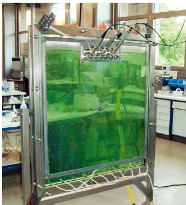
PLATE REACTORS WITH AN IDEAL LIGHT MANAGEMENT SYSTEM FOR CULTIVATING MICROALGAE. Photo: Florian Lehr, KIT
