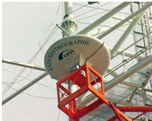
THE GEESTHACHT COASTAL RESEARCHERS' WAVE RADAR ON THE MEASURING PLATFORM FIN03. Photo: F. Ziemer, GKSS
