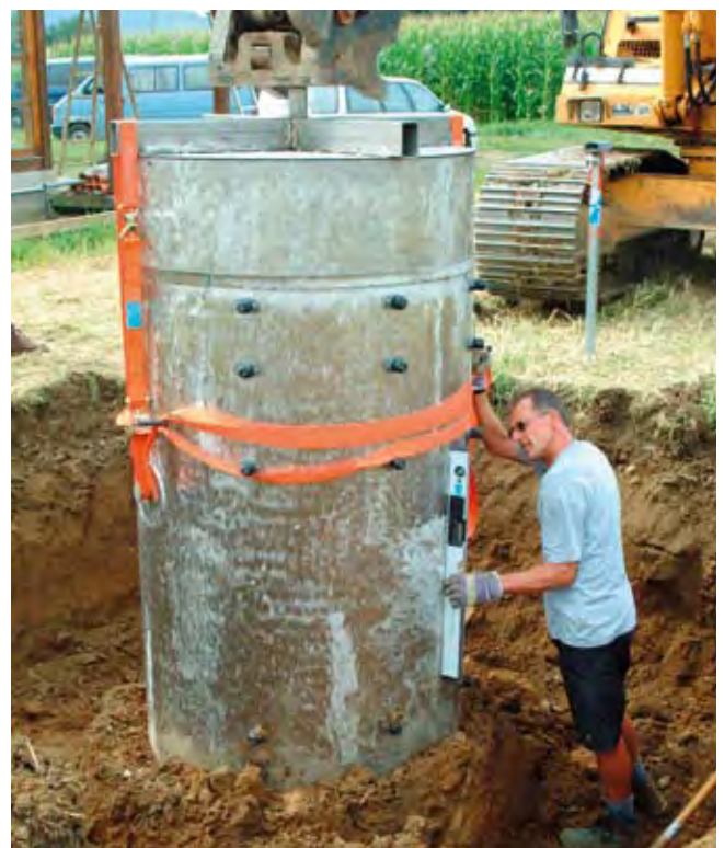
A LYSIMETER CONTAINS AROUND 1.5 CUBIC METRES OF SOIL AND NUMEROUS MEASURING DEVICES. Photo: Firma Umweltmonitoringsysteme
