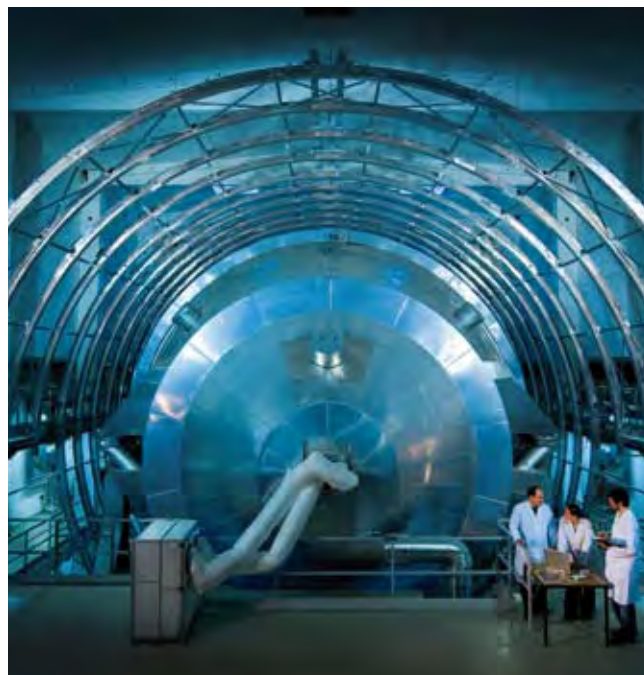
THE KATRIN SPECTROMETER IS SURROUNDED BY 15 LARGE RINGS WHICH BEAR THE COILS FOR GENERATING THE MAGNETIC GUIDE FIELD. Photo: KIT
