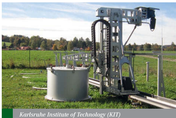
This robot, operated by KIT researchers, automatically measures nitrous oxide emissions from the soil. Image: E. Díaz-Pines
