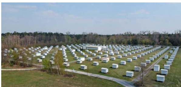
The KASCADE experiment uses 252 detector stations distributed over an area of 200 by 200 metres. Image: KIT
