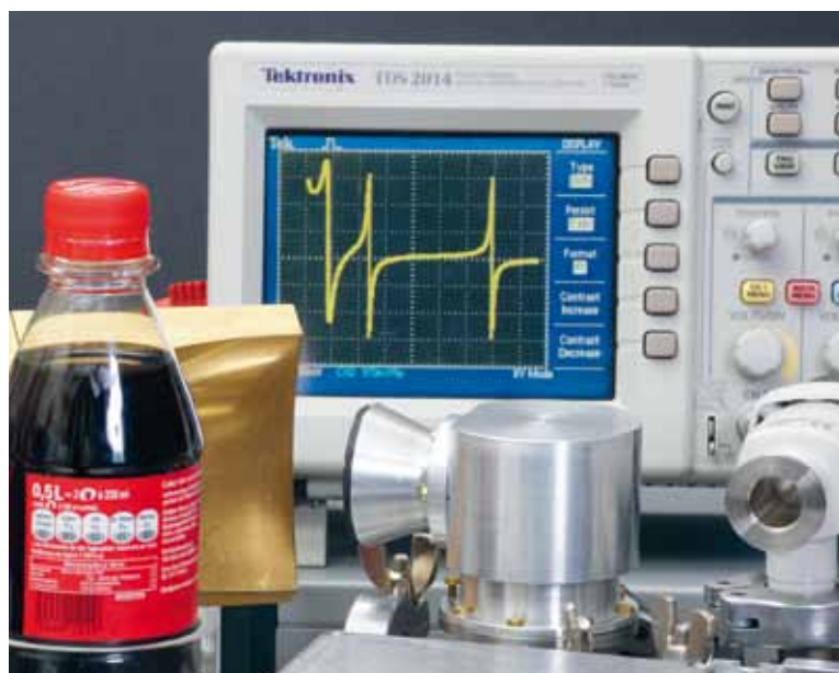
THE ASSEMBLY SHOWS THE PROTOTYPE OF THE DETECTOR (CENTRE) AND THE FLUID THAT IS TO BE EXAMINED IN A BOTTLE. THE LIGHT SOURCE IS LOCATED TO THE LEFT OUTSIDE THE PICTURE. Photo: Forschungszentrum Jülich
