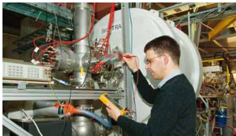
THE MASS OF THE ARTIFICIAL ELEMENT 102, NOBELIUM, WAS MEASURED WITH UTMOST PRECISION WITH THE ION TRAP SHIPTRAP. Photo: GSI/G. Otto
