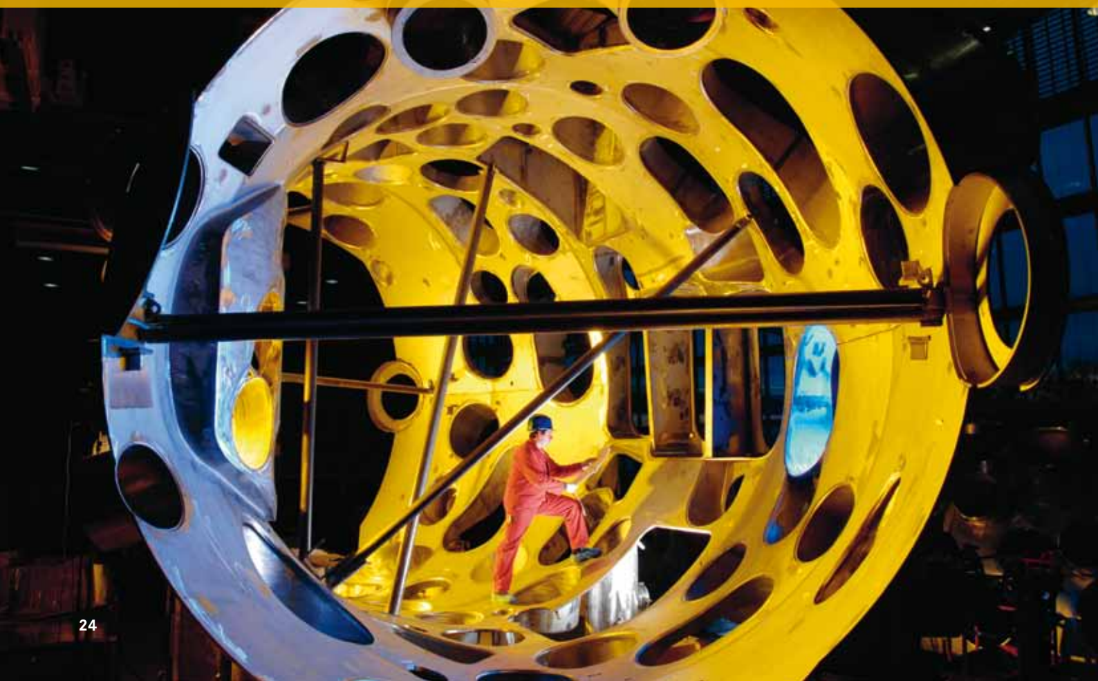
ONE OF THE FIVE PARTS OF THE OUTER VESSEL OF WENDELSTEIN 7-X. Photo: IPP/W. Filser
