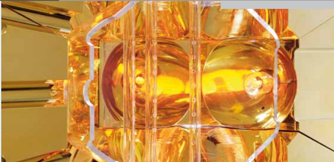
HIGH-TEMPERATURE MATERIALS, WHICH COULD IMPROVE THE EFFICIENCY OF POWER STATIONS, ARE RESEARCHED AND TESTED IN RADIATION FURNACES. Photo: FZJ
