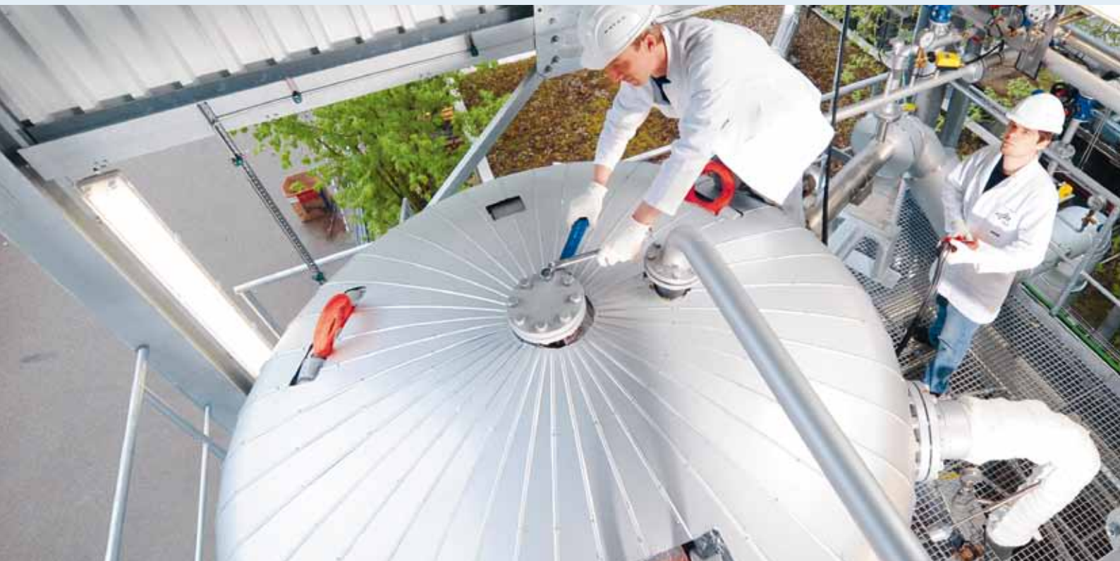
THE DLR EXPERTS HERE CAN TEST NEW CONCEPTS IN A VARIABLE STORAGE TEST UNIT WITH EXCHANGEABLE INNER CONTAINER. Photo: DLR
