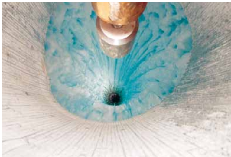
THE BORE HOLES FOR ICECUBE ARE MOLTEN INTO THE ANTARCTIC ICE WITH HOT WATER. Photo: J. Bolmont
