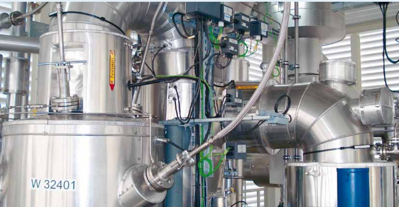
ON CAMPUS NORTH OF THE KIT, THE BIOLIQ PILOT PLANT WILL PRODUCE FROM STRAW AND OTHER RESIDUAL MATTER FIRST AN OIL-LIKE PRE-PRODUCT AND THEN FROM THIS TAILORED DESIGNER FUELS. Photo: KIT
