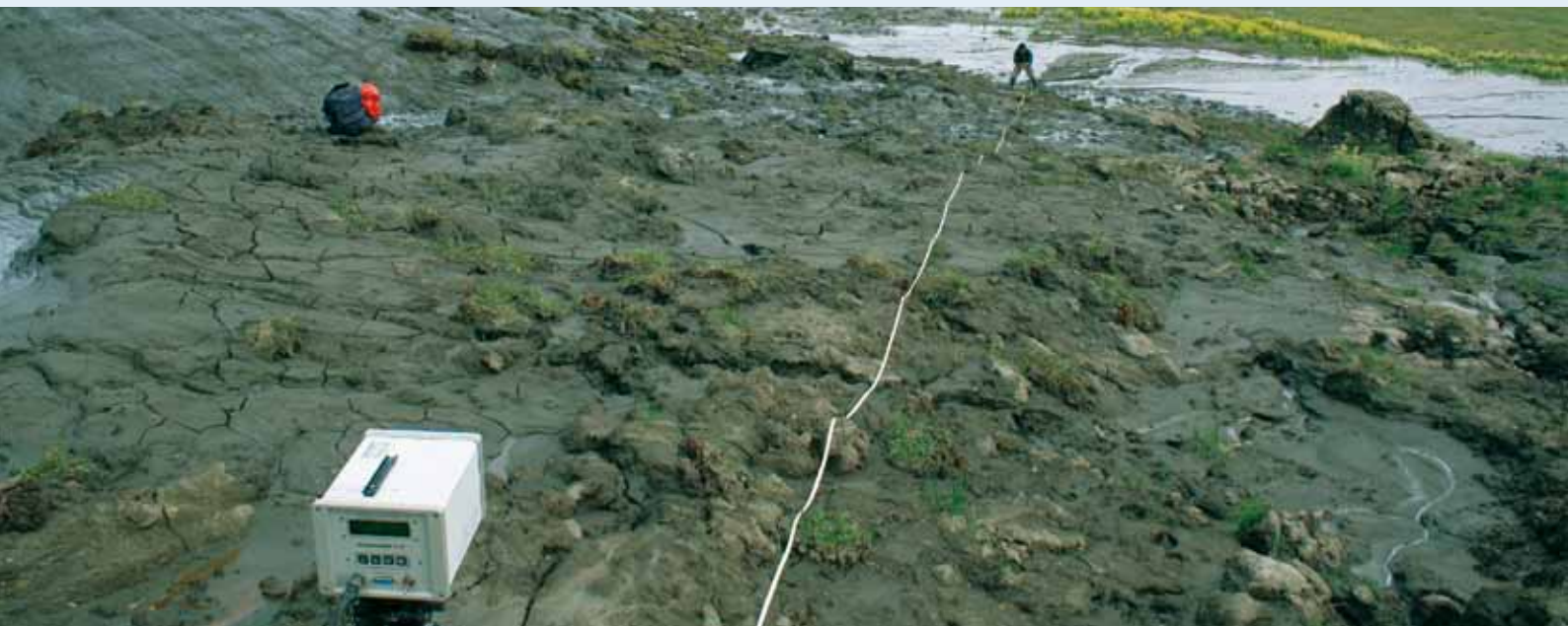
METHANE MEASUREMENTS AT A SO-CALLED THAW SLUMP ON HERSHEL ISLAND. THE THAWING OF THE ICE IN THE GROUND LEADS TO THE TRANSPORT OF SEDIMENT TO THE COASTAL AREA. THAWING LIKE THIS COULD BE A SOURCE OF BIOGENIC METHANE. Photo: GFZ/T. Sachs
