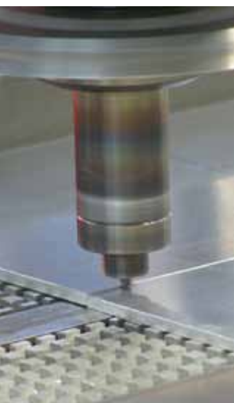
This new joining process, based on friction spot welding, is already in use in industry. Photo: HZG
