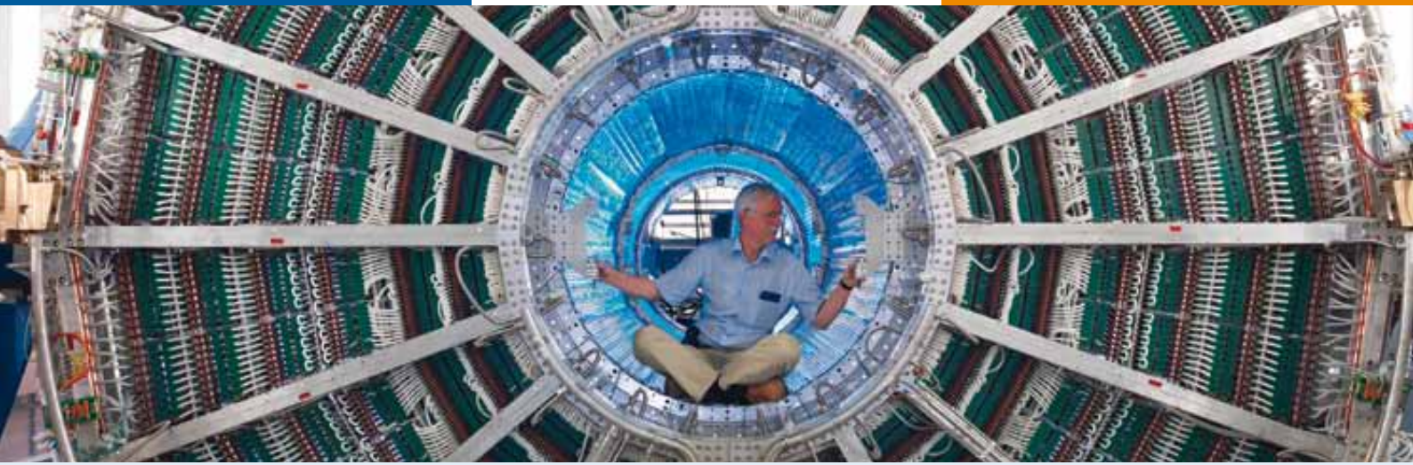
The TPC (Time Projection Chamber) is the component in ALICE that delivers the most data, producing extremely precise measurements of the traces of the generated particles. Peter Glässel, the technical coordinator of ALICE, is pictured here in the centre of the TPC. Photo: CERN
