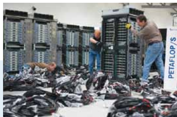
Experts assembling the JUGENE supercomputer, which has a computational capacity of one thousand trillion operations per second (petaflop), making it one of Europe's fastest computers. Photo: Forschungszentrum Jülich
