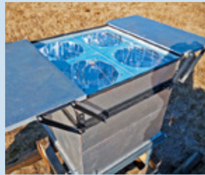
Figure 1: A Tunka-HiSCORE Cherenkov detector station, one of the nine stations operating since October, 2013 in Tunka. Design and construction were made in close collaboration between Russian and German groups. Image by DESY
