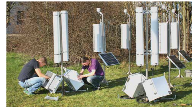
Researchers calibrate cosmic ray sensors in the Eifel-Rur observatory (TERENO) to measure the soil moisture content. © Heye Bogena, FZJ
