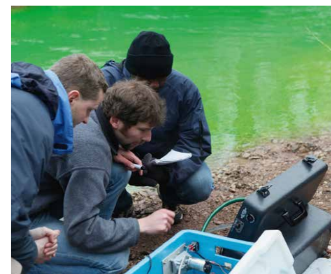
Researchers from the WESS research cluster study the exchange processes and transposition rates of solutes in the hyporheic zone using hydrological tracer substances in the Bode catchment. © Hermann Rügner, University of Tübingen
