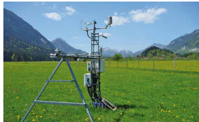
The TERENO pre-alpine hydrometeorological test site in the Ammergau Alps: measuring energy flow using the eddy covariance technique. © Harald Kunstmann, KIT
