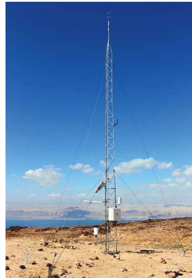
Meteorological measuring tower in the west of Madaba (Jordan). The Dead Sea is in the background. Researchers have been measuring wind speed, wind direction, air temperature, relative humidity, short-wave and long-wave net solar radiation, air pressure, rainfall, soil heat flux and soil moisture since March 2014. © Friederike Lott, KIT
