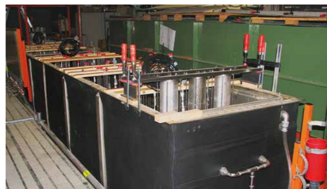
Inputs of harmful substances and their degradation speeds in groundwater are being analysed by researchers in the artificial indoor aquifer at the Helmholtz WasserZentrum München (HWZM). © Tillmann Lüders, HMGU
