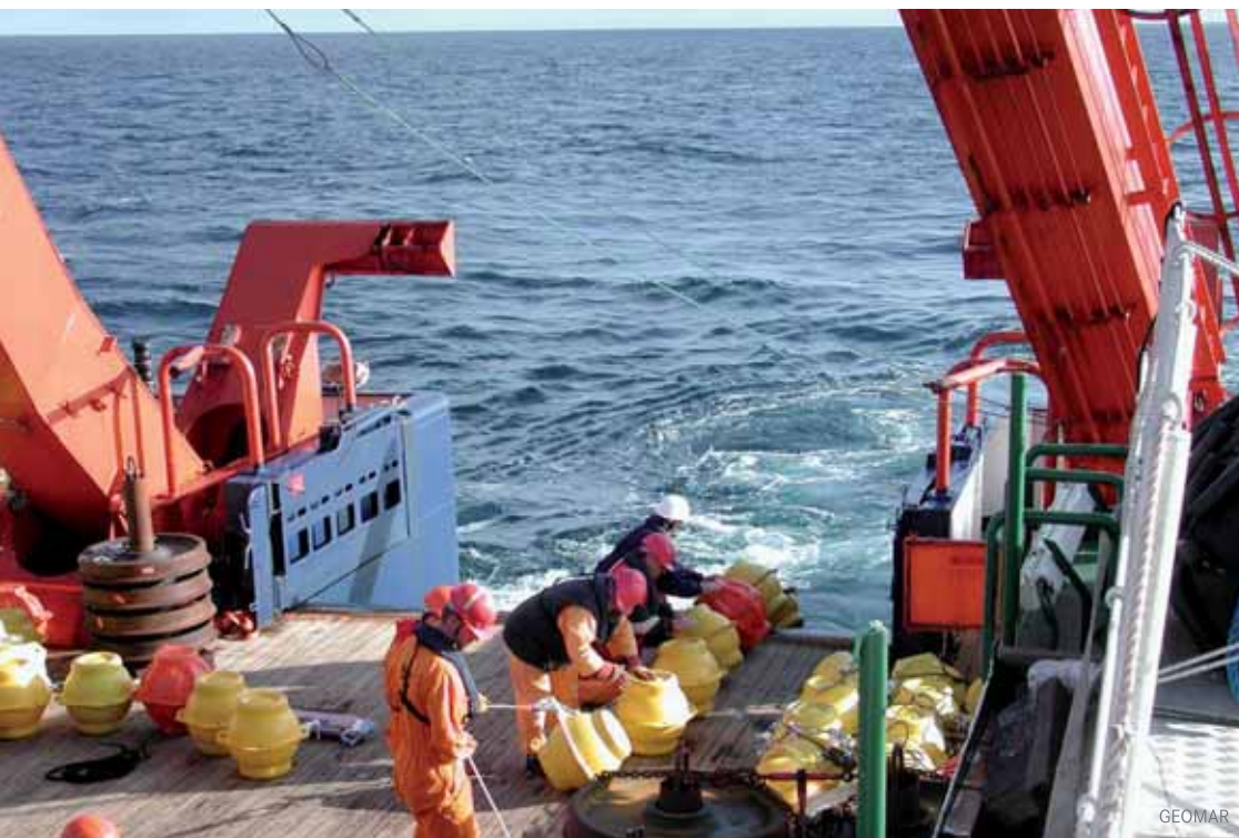
Deployment of the central deep sea mooring in the Labrador Sea MOC Array with the global ocean Research Vessel "Meteor". Bouyant glass spheres capable to withstand the immense pressure of the deep ocean are used to keep the mooring wire upright and the instruments in their target depth. This operation is repeated bi-annual.
