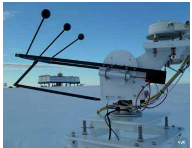
Antarctic base Neumayer III and instrumentation for measuring surface radiation balance.
