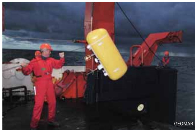
Early morning deployment of a Moored CTD/Velocimeter Profiler (MVP) in the Labrador Sea MOC Array. This instrument is motor-driven for climbing the mooring wire up and down. The internal battery has sufficient energy for traveling 1 Million Meters (i.e., 1000 profiles of 1000m length).
