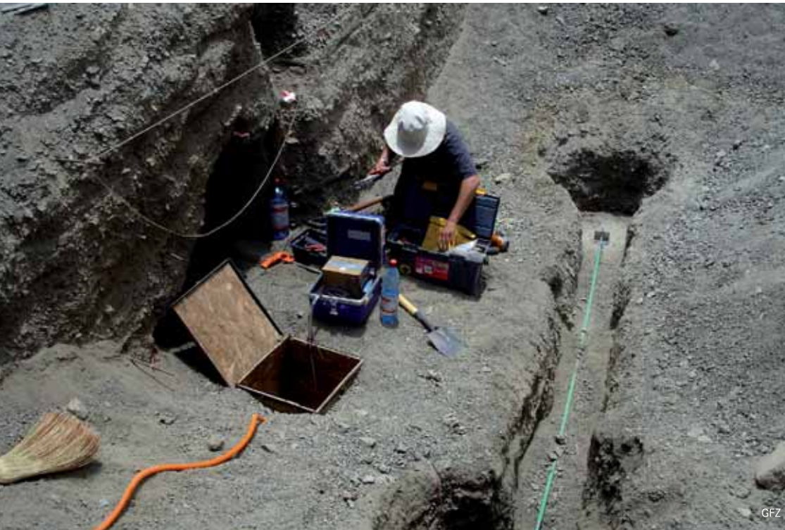
Installation of a Creepmeter station of Chilean plate boundary observatory IPOC in the Atacama Desert, Northern Chile.
