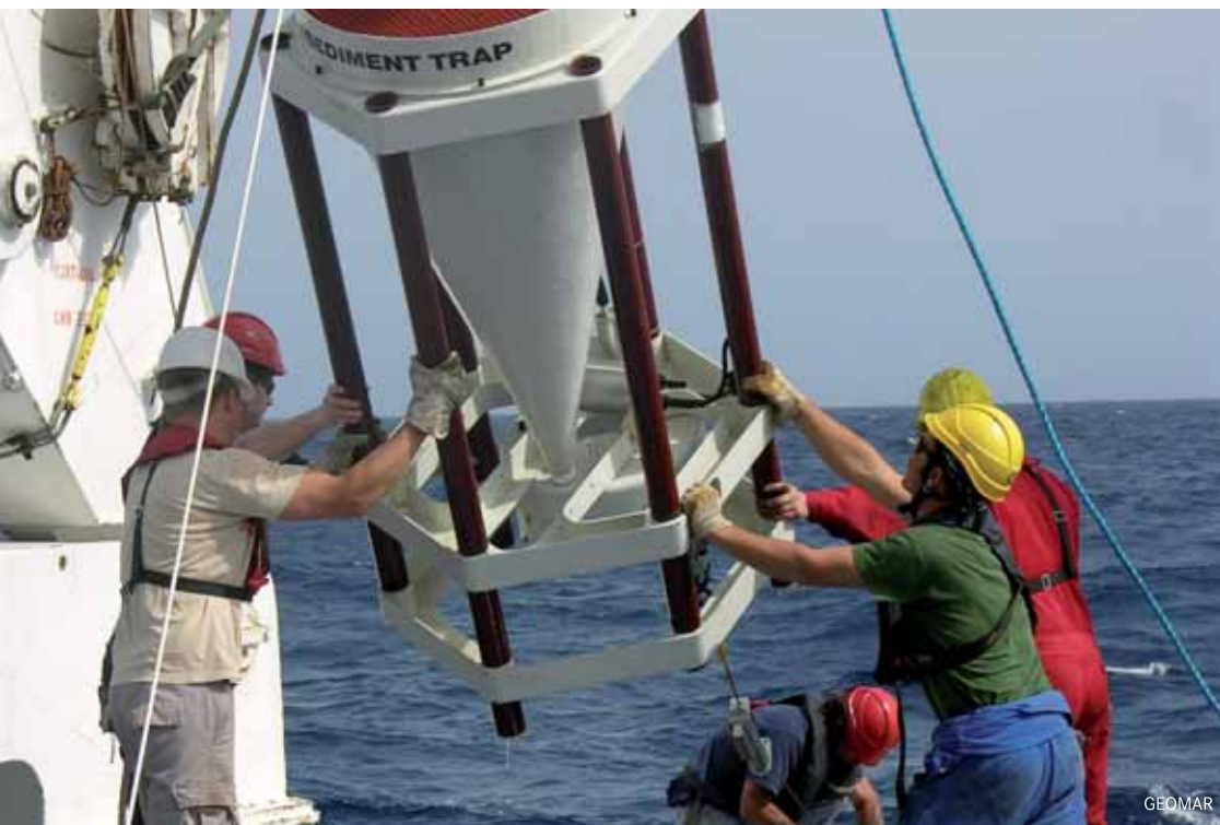
A Sediment trap to investigate chemical and biological processes at the Cape Verde Ocean Observatory. This Trap is incorporated in the moored CVOO-station which is serviced (recovered and deployed) in an annual to bi-annual rhythm. This station measures a suite of physical and biogeochemical parameters.
